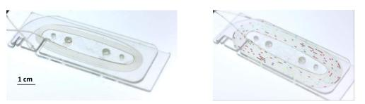
Left: Empty storage coil made of FEP tubing of 0.8 mm OD. Right: Nanoliter volume sequenced droplets ready for push/pull operation.
