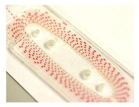
A Droplet Storage Coil with ~ 450 reactions in a 3 inch<sup>2</sup> area. The fluid flow rate sets the bounds of throughput.
