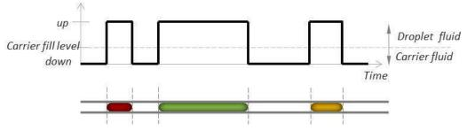
'Up' and 'down' Motion of the sampling nozzle controls droplet size and carrier spacing.
