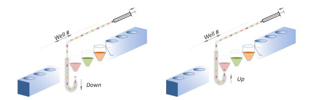
Schematic showing Dropix®Sample Hook assembly motion relative to the Sample Strip. Left: In 'down' position aspirating carrier fluid. Right: In 'up' position aspirating droplet fluid.
