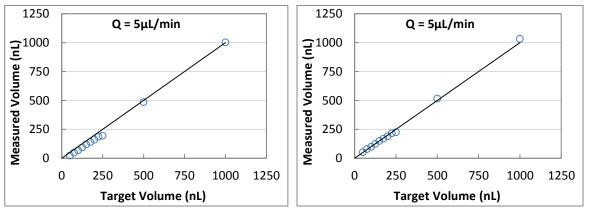
$Q = 5 \mu L/min$ . Left: Uncalibrated. Right: Calibration with offset = 30 nL.
