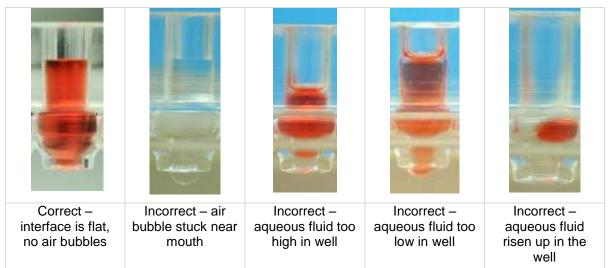
A: The aqueous fluid should rest at the mouth of the wells as in the image to the left. To the right, a well is seen with an air bubble lodged, a pendant droplet hanging, or with a receding interface – these are undesirable and require corrective action. Adjustment with a micropipette evens out the hanging drops. There should be no air bubbles visible at the
