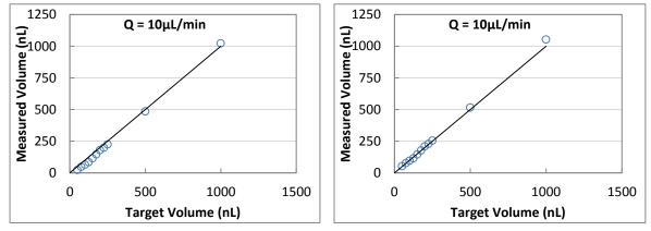
$Q = 10 \,\mu$ L/min. Left: Uncalibrated. Right: Calibration with offset = 30 nL.
