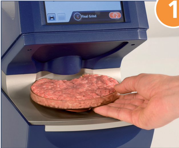
Place prepared sample in sample holder
