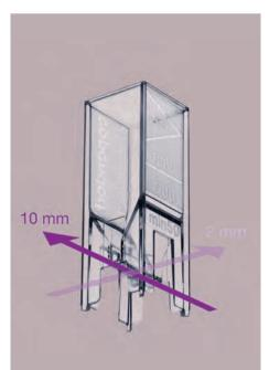
The patented\* Eppendorf UVette is a fully UV-transparent, single use cuvette made of clear plastic, with a light transmission of 220 nm to 1,600 nm. The unique design allows you to conduct flexible measurements with two different light paths (10 mm and 2 mm).
